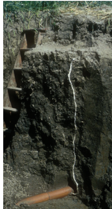
Figure 3 Lumbricus terrestris burrow ending on tile surface. At its end the burrow bends towards the tile. The plough layer has been removed and the cast starts from a depth of approximately 0.25 m. The tile is at a depth of 1.0 m. (from Nuutinen & Butt, 2003).
